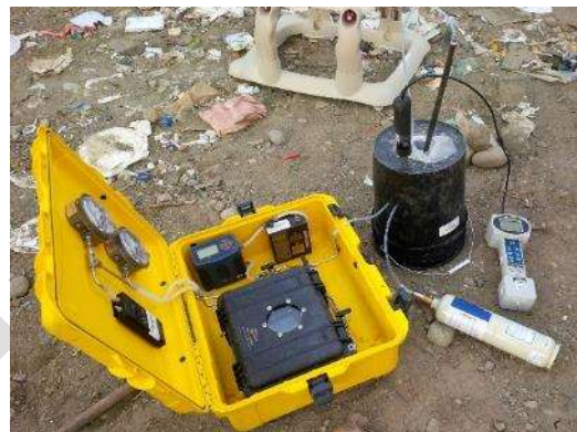
Figure 13: Leak testing drive-point soil vapour probe at a SDWDS near Lillooet, British Columbia
