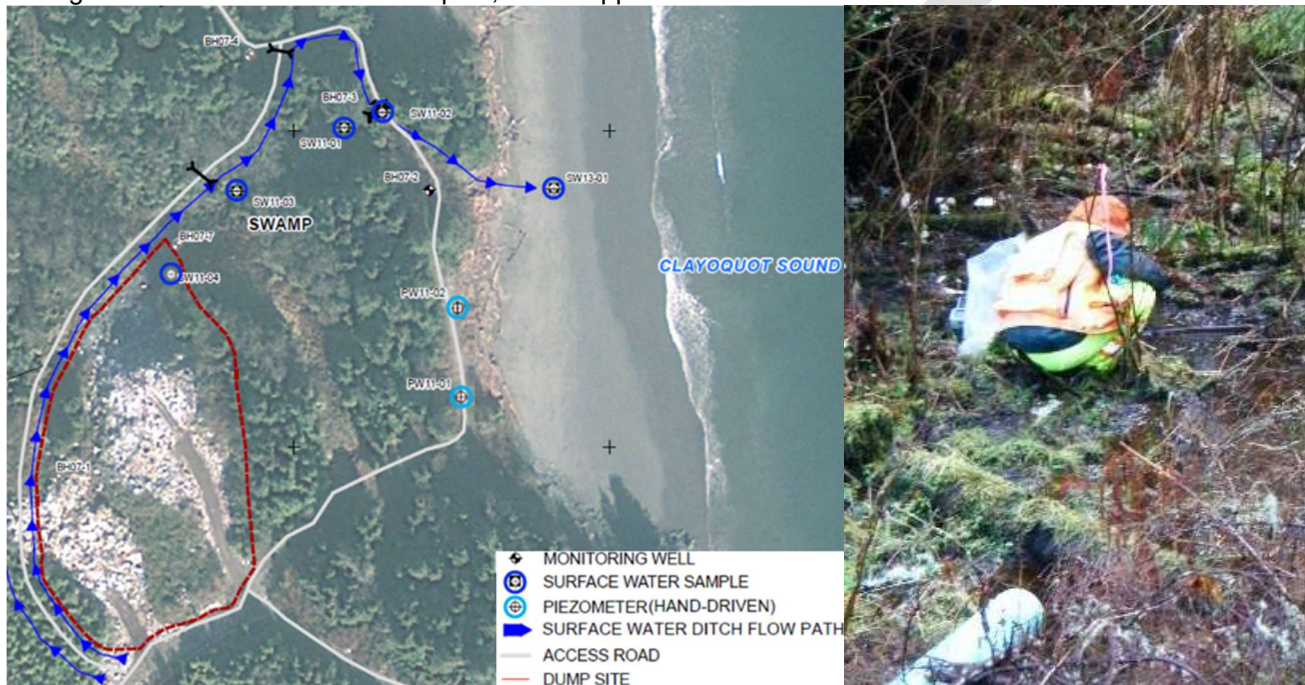
Figure 15: Surface water quality sampling plan for a SDWDS in Ahousaht, British Columbia (left) and surface water quality sampling at depicted Site location SW11-02 (right)
