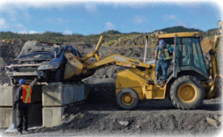
An end-of-life vehicle is placed on a platform of lock-blocks to enable safe access to the underside.
