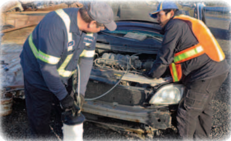
Brake fluid is drained using a hand pump.
