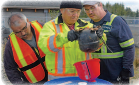
Recycling expert David Peaire (right) watches as Roger Vickers drains the oil from the fridge compressor into a storage drum.
